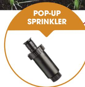
Pop-up sprinklers are designed to distribute water evenly over lawn surfaces. The spray mimics a soaking rain. Pop-ups normally have 15mm inlet threads and come with variable arc nozzles or fixed spray nozzles. Both have various throw characteristics. Pop-ups should be placed evenly apart with the spray reaching from the head of one sprinkler, to the head of the next sprinkler. This ensures full coverage and no dry spots.
